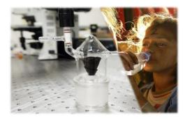
A new device for collecting and purifying water, developed at The University of Texas at Austin, was inspired by a rose and, while more engineered than enchanted, is a dramatic improvement on current methods. Each flower-like structure costs less than 2 cents and can produce more than half a gallon of water per hour per square meter.
